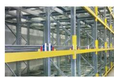
Pallet rack in empty condition, all trolleys are on top of each other on the storage side
