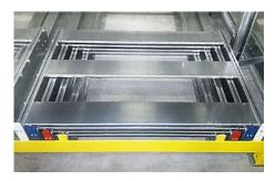
All three pallet runners are supported in the "Pushback Trolley System". As a result, even damaged pallets can be reliably stored regardless of the pallet quality.
